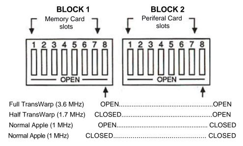
Figure 2 Sample Switch Configuration for Apple //e System
