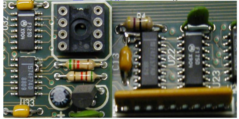
We also recommend replacing the old Electrolytic Capacitors on the TransWarp GS board. They are now well past their designed lifespan. This will help ensure that power issues are kept in check as originally designed. We will be offering this upgrade service in our <u>Store</u> soon. Email <u>Support</u> in the mean time if an upgrade is desired.
