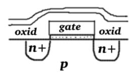
In the picture there are areas with n+ additives on a p type carrier; among them a thin oxide layer on silicon (see dotted a on top of it polycrystal silicon. All this is covered by an oxide layer and a protective layer. The two n+ areas are the So and Drain electrodes of the transistors (their sequence is insignificant here as the structure is symmetrical); the polysilico Gate electrode.
