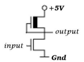
The essence of the operation of the inverter as a two-transistor switch is whether the lower (driver) transistor pulls dow output to 0 potential or not. This depends on the input. If the input is logical 1 (e.g. 5V), the driver opens, that is, it for short circuit between the output and the ground; thus the output becomes logical 0.
