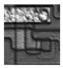
In the end, the last configuration needed to analyse the nMOS layout: depletion mode transistor. This type of transistor c found in every logical gate. Its gate is always connected to its Source electrode and the Drain is connected to the possupply. In this layout the aluminum wire is +5V, and the gate is reconnected to the Source through a buried contact.
