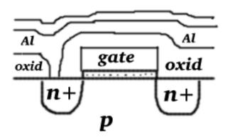
Let us now take the aluminum wire into the cross-section picture. The oxide layer above one of the electrodes is interrulthere is a passing through the transistor-electrode and the aluminum wire. The aluminum wire and the polysilicon wire each other without any pass over; this is impeded by the oxide layer.
