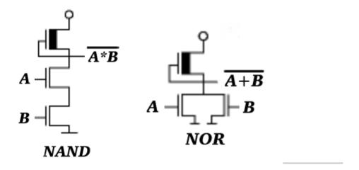
There are so-called complex gates too, with multiple inputs connected in series and in parallel, the functioning of the easily be deduced by the NAND and NOR logic.
