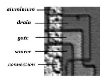
The light grey vertical wire is the aluminum, which crosses the transistor and is connected to the Source electrode through a contact. The circular area is the contact with an active zone under it, but this can only be deduced from the zone boundary, from the colour. Sometimes it is difficult to analyse such areas, which are covered by large-surface metal layer.
