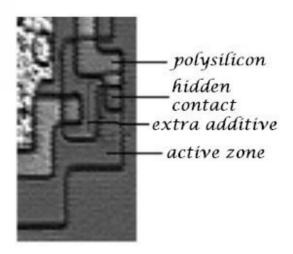
There is another type of contact, the hidden one, which provides a pass over between the active zone and the polysilicon. extra additive is used to avoid the rectifier feature of such a transition; this can be observed in the layout photo.
