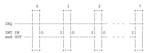
The system was designed so that if INT IN for a slot is low then that slot may not generate an interrupt. Each slot should pull INT OUT low when it is requesting an interrupt to disable lower priority slots. Cards that don't use IRQ should wire INT IN and INT OUT together so that any higher priority slots can still disable cards in lower priority slots. This priority system fails if there is an empty slot between any two interrupting cards.
