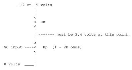
The voltage range at the GC inputs should go from 0v to 2.4v. The value of Rs can be calculated for +5 volt systems with this formula:
