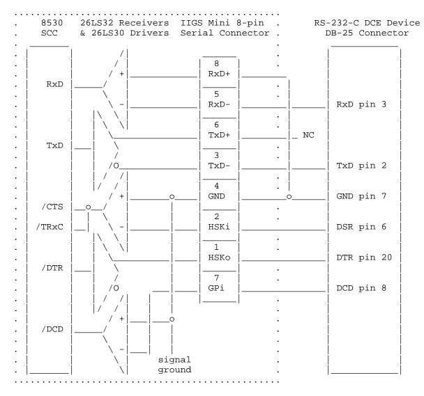
Figure 7-x2-Apple IIgs Connection to an RS-232-C DCE Device
