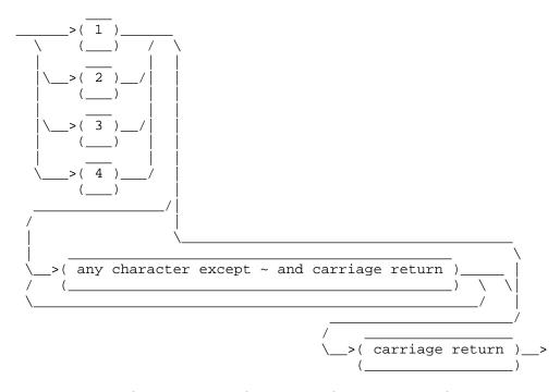
Figure 12-requiredFlag Field Syntax Diagram
