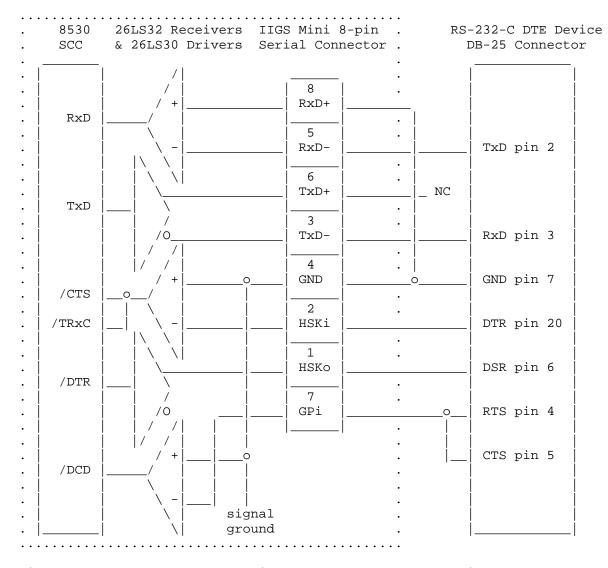
Figure 7-x1-Apple IIgs Connection to an RS-232-C DTE Device
