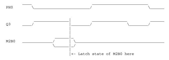
Figure 1-When to Latch State of M2B0
