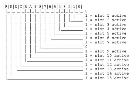
Figure 2-Bit Encoded Slot Configuration
