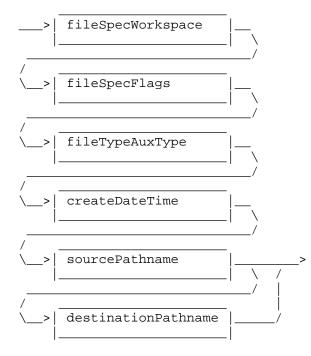
Figure 9-fileSpecification Field Syntax Diagram
