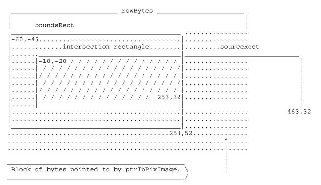
Figure 3-Sample LocInfo Structure Offset by -60,-45
