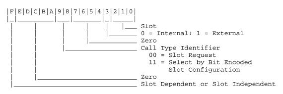
Figure 1-Slot Number and Bit Definitions
