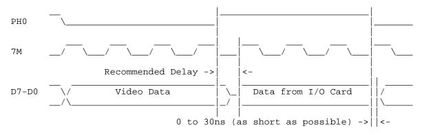
Figure 3-Recommended Data Transfer Timing
