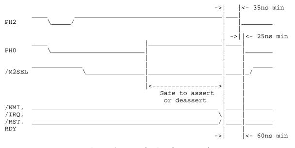
The RDY line should be driven with an open-collector driver.
