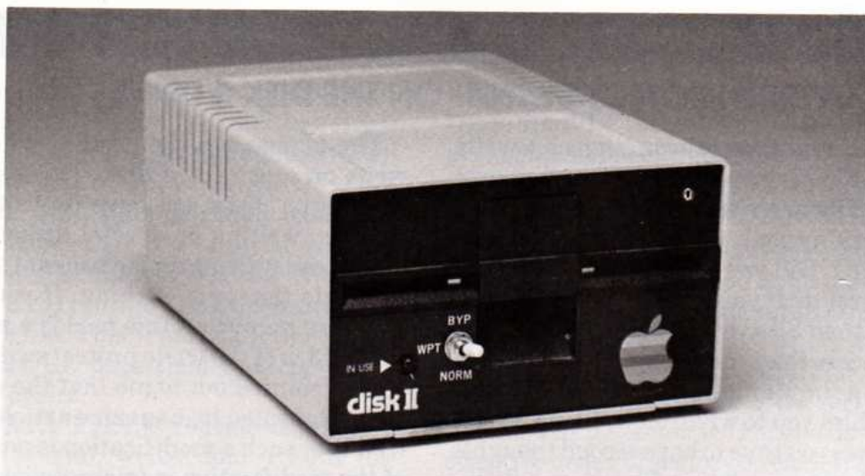
Figure 9.22 A Drive With the Write Protect Switch Installed.
